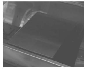
Insert the drip pan with the long edge on the left. Ensure the drip pan is sloped down from right to left.
