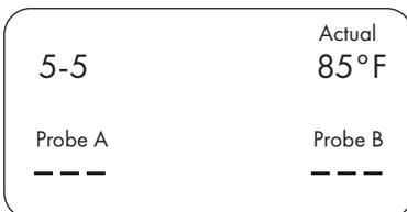
**Screen 5-5** is test mode for your grill's temperature sensor and Probe A and Probe B. You can see the temperature values for each displayed on the screen (a value of - - - means the probe is not plugged in or the grill's sensor is not connected).
