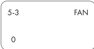
**Screen 5-3** is test mode for your grill's blower fan. You should be able to hear the fan blowing.
