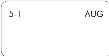
**Screen 5-1** is test mode for your auger motor. You should be able to look in your grill's fire pot and see the end of the auger turning very slowly.
